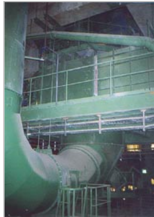
Lower part of the air separator VTP 2900 with exhaust duct at the cement grinding plant for 130 t/h at Anhovo, Slovenia
