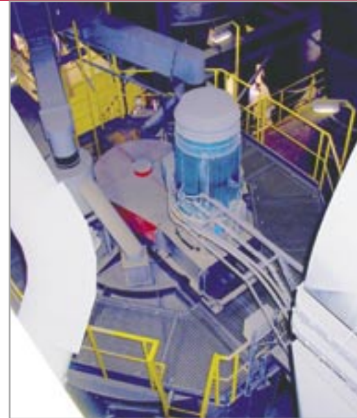
Air separator VTP 2700 at the cement grinding plant with a capacity of 80t/h – CEMMAC Horné Srnie, Slovakia
