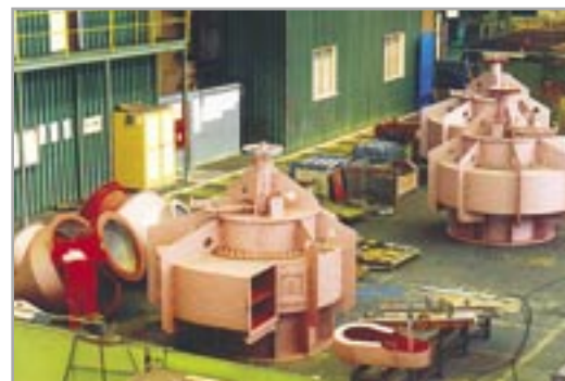
Assembly of VTP 1500 air separators for a cement grinding plant in Brazil
