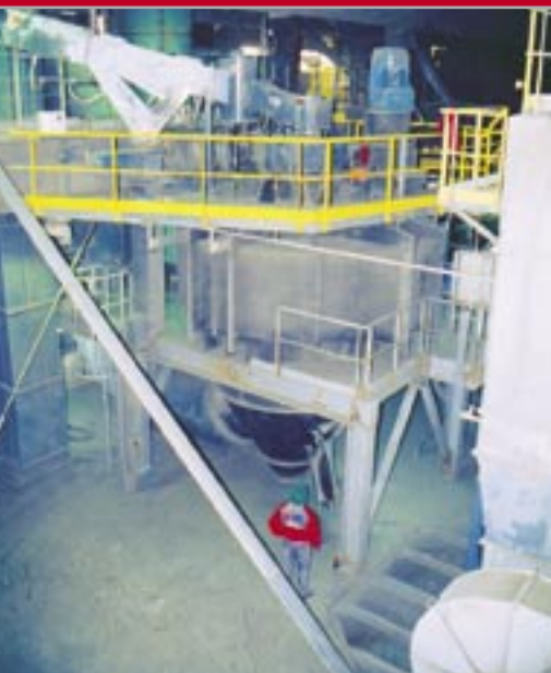
Air separator VTP 2400 at the cement grinding plant with 100t/h capacity – Kujawy, Poland
