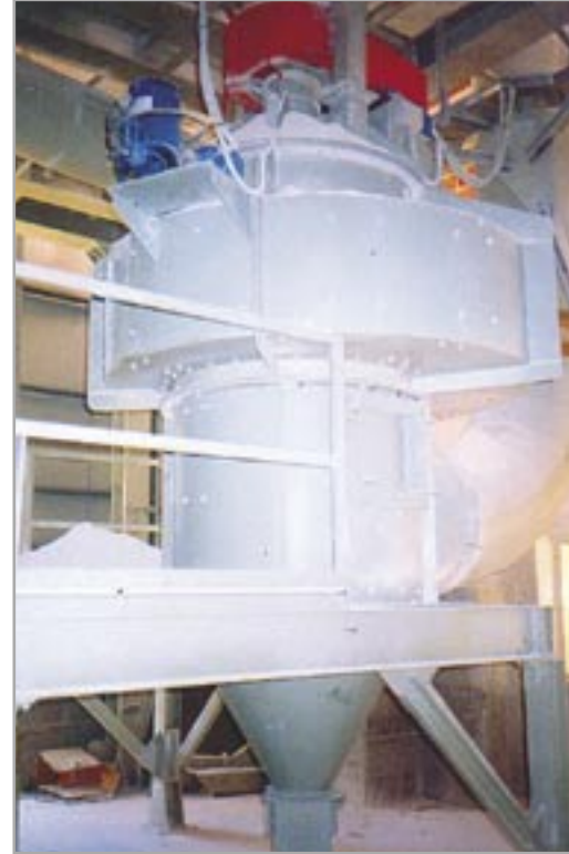
Air separator VTP 1100 at the limestone grinding plant for 9 t/h at Redipuglia, Italy
