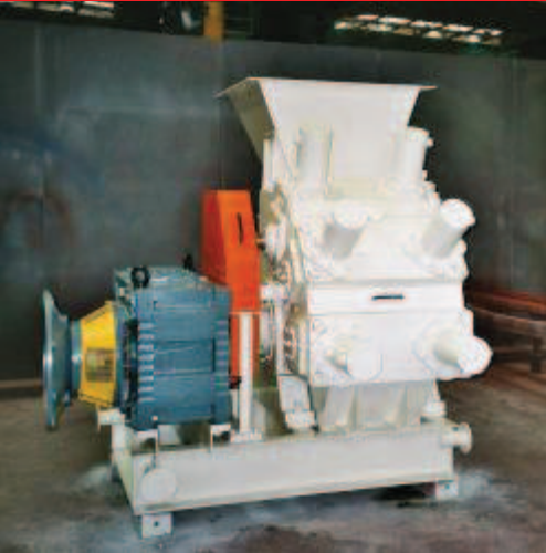
Horizontal roller mill PREMILL PM 800
