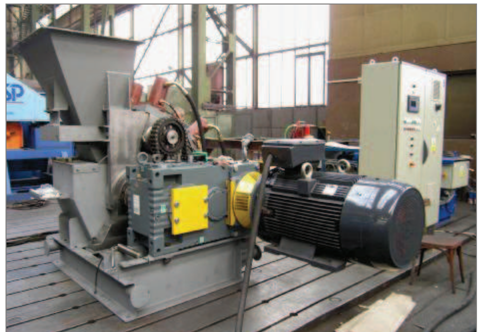
PREMILL PM 800 in the test facility of PSP Engineering
