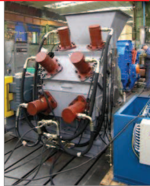
PREMILL PM 800 at the workshop PSP Engineering for limestone grinding at Vitošov, Czech Republic
