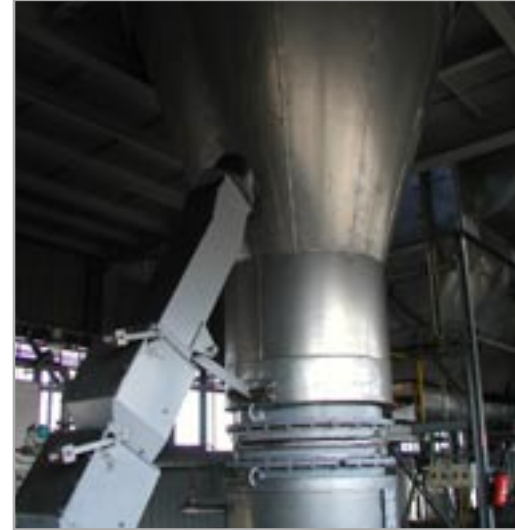
Air separator LTR-R 1650 at the coke grinding plant with 12.5t/h capacity – OKD Ostrava, Czech Republic
