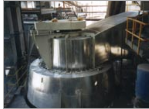
Air separator LTR-R 2500 at the cement raw material grinding plant with a capacity of 105t/h – Rezola, Arrigoriaga, Spain
