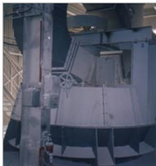
Air separator LTR-R 2000 at a lime grinding plant with 36 t/h capacity – Vitošov, Czech Republic
