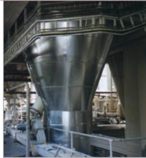
Air separator LTR-R 2500 for 105t/h at the cement raw material grinding plant – Rezola, Arrigoriaga, Spain
