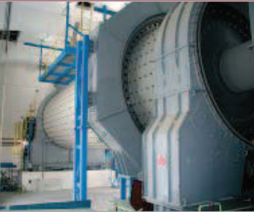
Cement grinding plant with a \varnothing 4.0 x 13.75 m mill seated on shoe-type bearings
