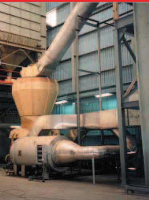
Grinding plant with the KTM 1600 for ceramic material. (UAE)
