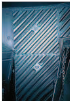
Detail of the grinding chamber armoring
