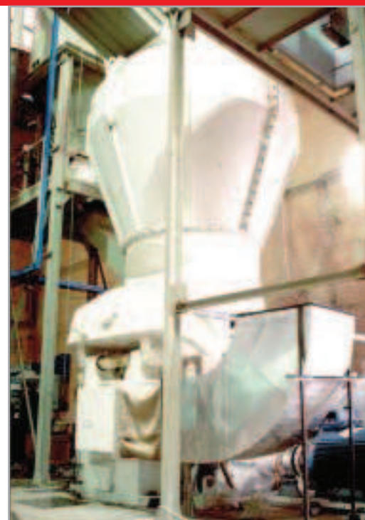
Assembly of a KTM 1600 for grinding material used for floor and wall tiles.
