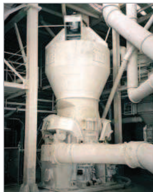
Reconstruction of a KTM 1400 with a DTIM 1500 separator
