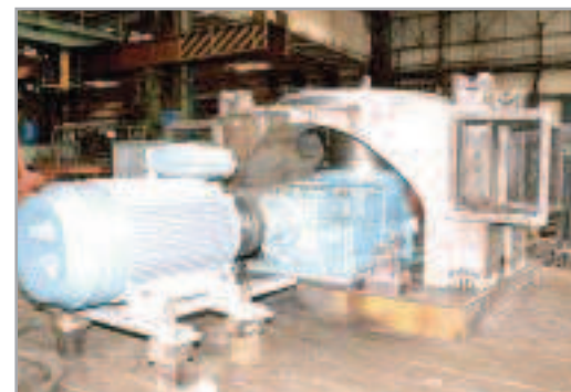
Electric motor with gearbox
